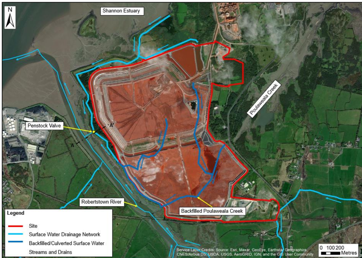
Figure 10.9: Surface Water Drainage associated with the BRDA Aerial Photo Source – Bing Maps (2013)
