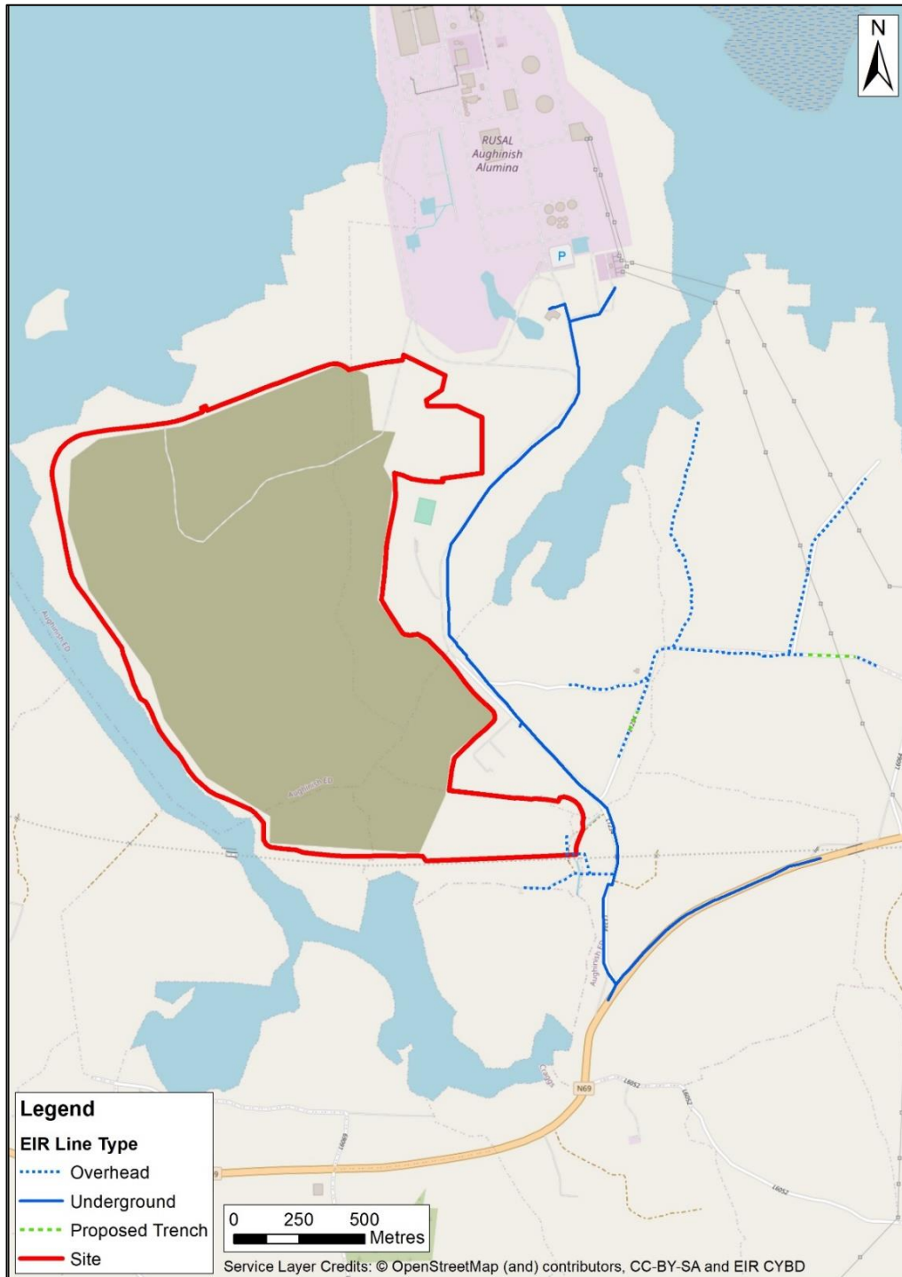
Figure 15.5: Eir Service Layout surrounding the Application Site
