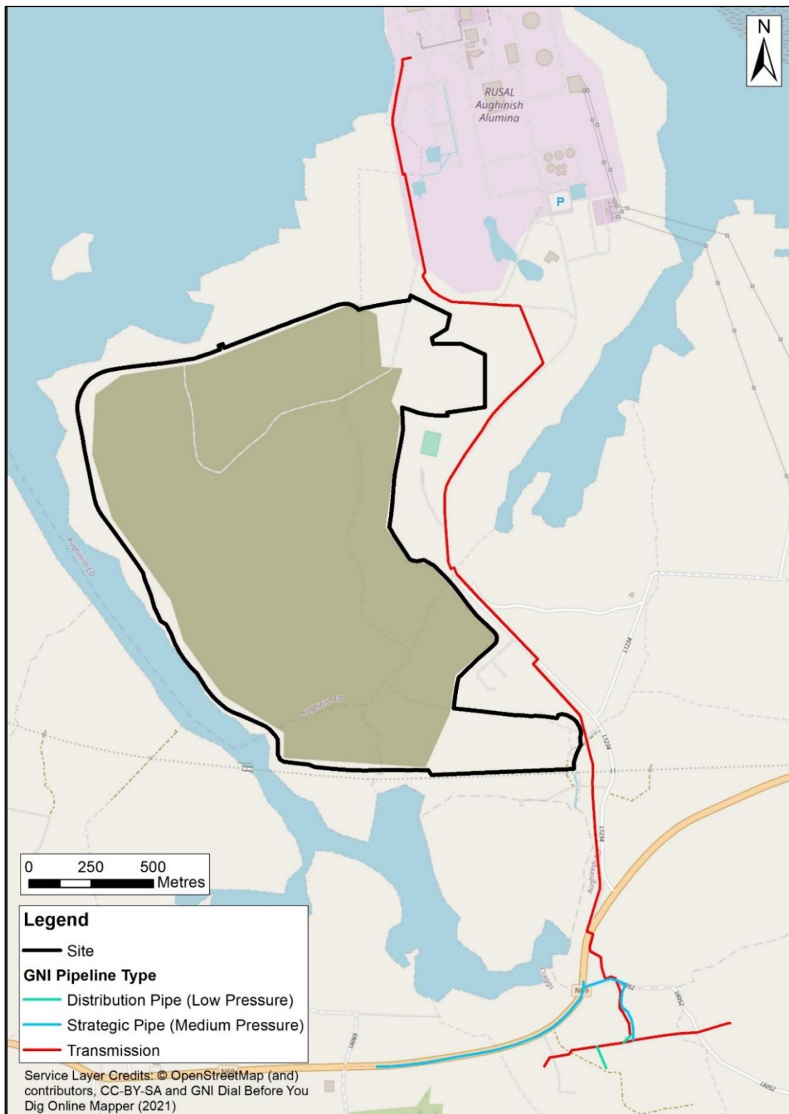
Figure 15.4: Gas Supply near the Application Site
